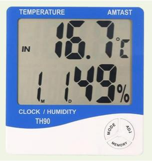
A thermo-hygrometer is an instrument used to measure and display both the temperature and relative humidity of the surrounding environment.
